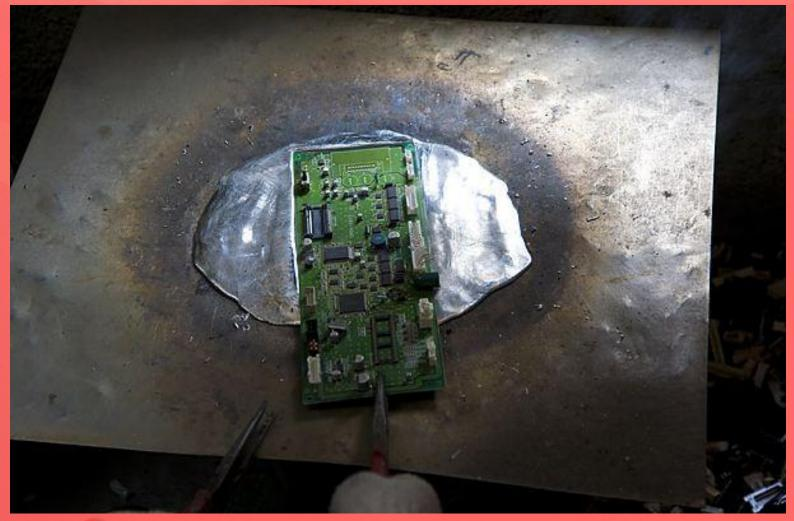
The ewaste is mined for the lead, gold, copper and other metals that are found in the circuit boards, wiring, chips and other parts of electronic devices. In this photo, a worker heats a computer board on a steel surface to remove the computer chips soldered into it.
